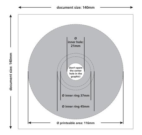
The grey area from 21-116 mm in diameter is printable!
